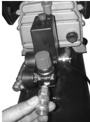
Figure 4. Installing the Air Chuck
